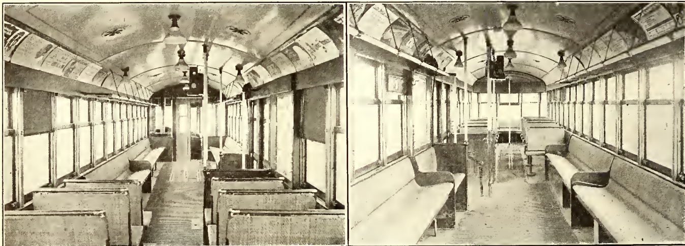
INTERIOR VIEWS OF THE FRONT-ENTRANCE, CENTER-EXIT CAR NOW IN USE IN TRAIN OPERATION IN TOLEDO, OHIO
